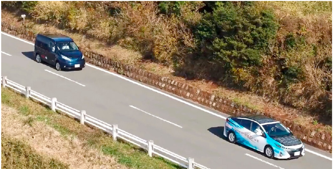
Fig.28 - PV-powered vehicles driving on public road in Japan (photo: courtesy of New Energy and Industrial Technology Development Organization (NEDO), Japan) PV-powered vehicles with around 1kWp PV integrated into the passenger vehicles were developed under the NEDO project in 2019/2020. Since then, these vehicles have been performing demonstration driving for data measurement and performance verification on public roads in Japan.
