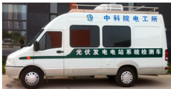
Fig.10 - PV plant inspection vehicle using modular test equipment for on-site performance testing of PV power plants in China.
