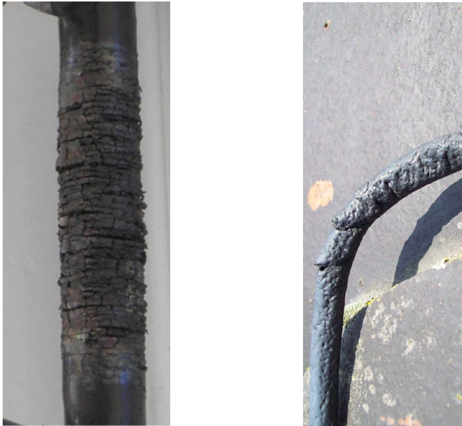
Figure 26: Examples of damages in cables in power plants located in the Atacama Desert.
