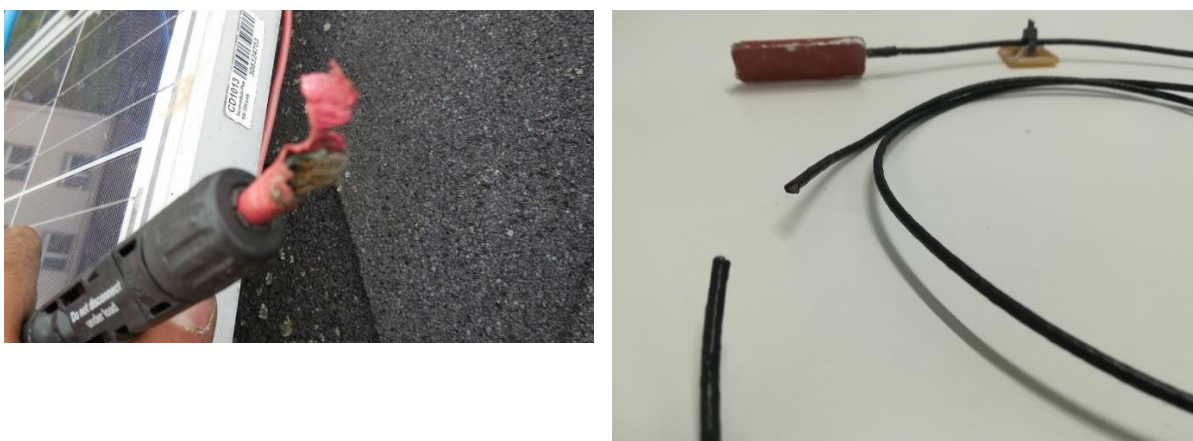
Figure 12: Cable bitten by a marten (left) (pveurope.eu © Leitl). Temperature sensor cable cut in half by a rodent (right) [Eurac Research].
