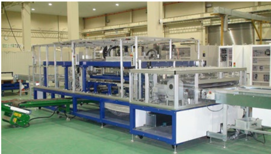
Fig. 3.4 Module delamination, i.e., glass and EVA separating equipment (Photo courtesy of NPC Incorporated)
