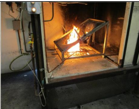
SBI test "variant" for PV roofs.
