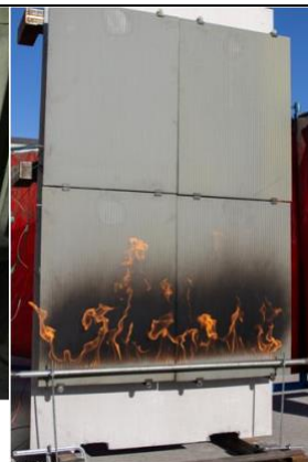
PV façade with Rapid Shutdown System – outdoor scoping test.
