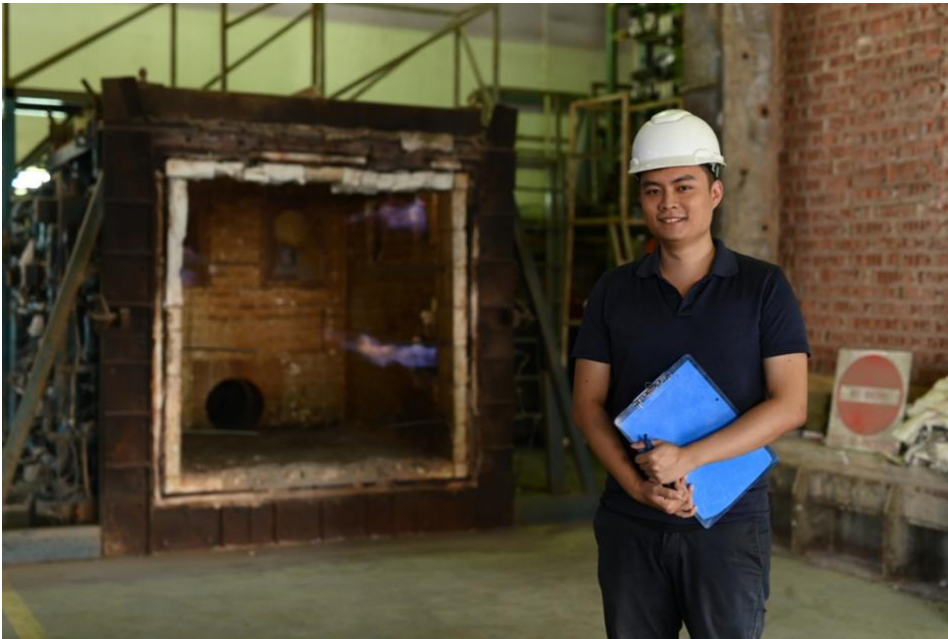
Figure 26: Furnace for fire-resistance testing.
