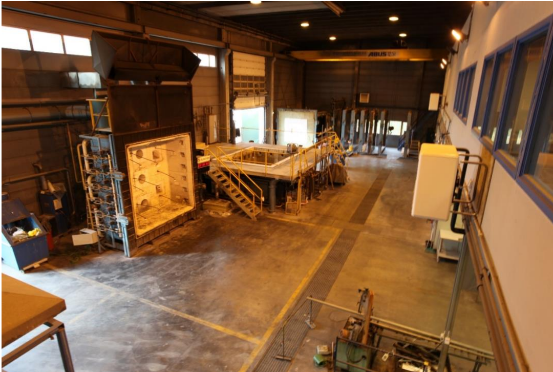
Figure 13: Test apparatus for reaction to fire test of external fire exposure to roofs (CEN TS 1187). Photo credit: RISE Fire Research.
