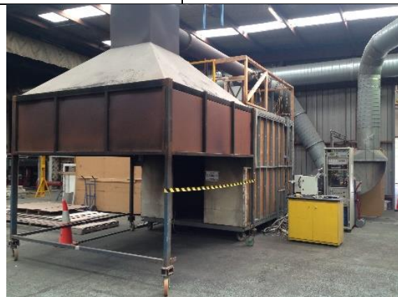
Photo of the ISO 9705 test rig.
