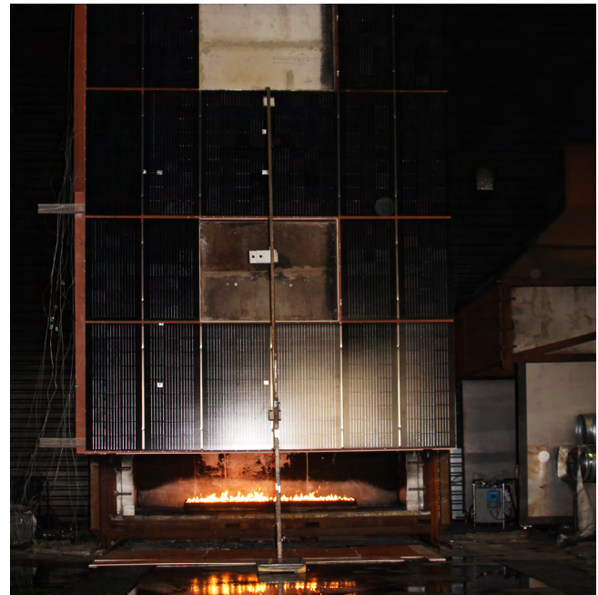
Fig. 23- Reaction to fire test according to method SP Fire 105 on a BIPV façade system. (Source: RISE Fire Research).
