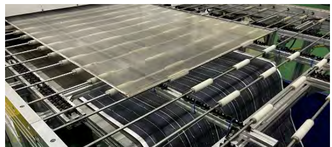
Fig. 7 - Separated materials after the hot knife technology (Photo courtesy of NPC Incorporated)
